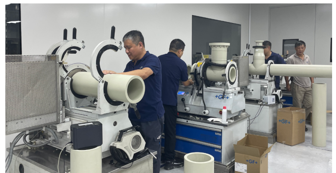
GF Piping Systems successfully combined the efforts of four of its major prefabrication facilities to provide over 1,000 easy-to-install PROGEF spools.
